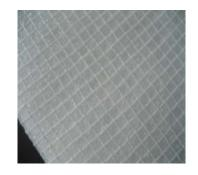
The wind surface of the meshes specially compact, and also put a fishing net to strengthen it; this structure make the filtering material keep the high filtering efficiency and large dust holding
